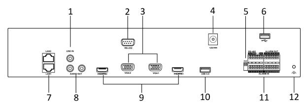
Figure 1-15 iDS-6700NXI-I/8F(B) Series Rear Panel
