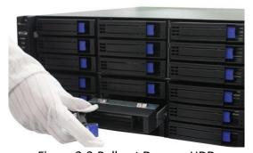
Figure 2-3 Pull out Dummy HDD
