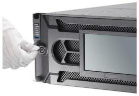
Figure 2-1 Unlock the Panel
