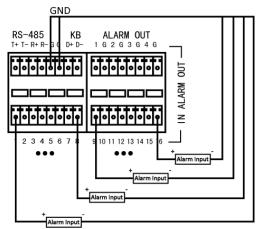
Figure 2-15 Alarm Input Wiring
