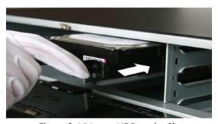
Figure 2-14 Insert HDD to the Slot
