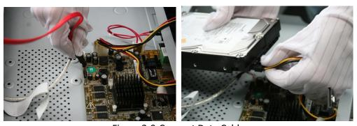
Figure 2-9 Connect Data Cable
