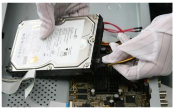
Figure 2-10 Connect Power Cable
