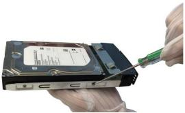
Figure 2-4 Fix the Hard Disk
