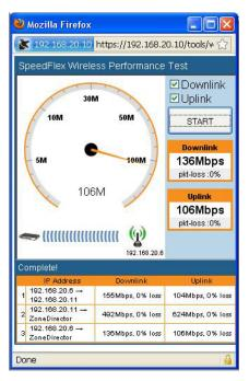
SpeedFlex™ is a unique wireless performance test tool integrated within the ZoneFlex™ family of centralized controllers that measures the Wi-Fi throughput of associated wireless LAN clients.
