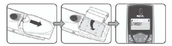
Replace the battery cover by sliding it back into place.
