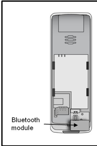
**Figure 22: Bluetooth module removed**
