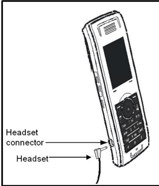
**Figure 18: Connecting the headset**
