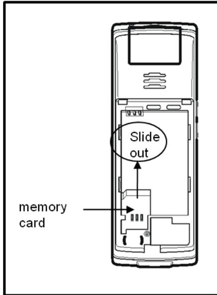
Figure 20: Removing the MEM card
