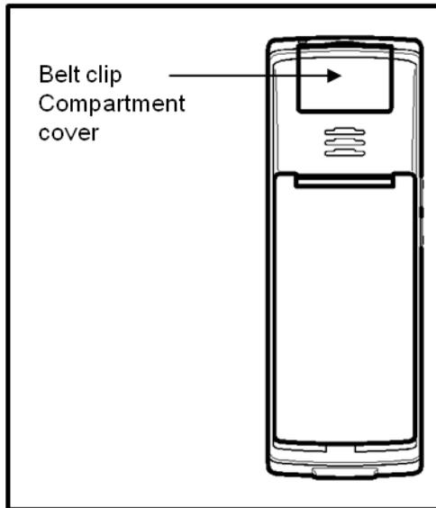
**Figure 17: Installed belt clip compartment cover**
