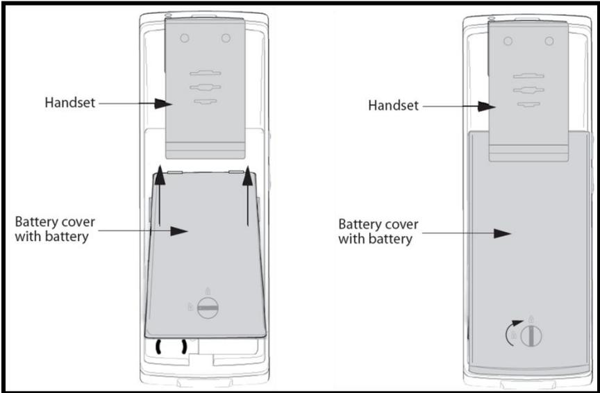
**Figure 2: Installing the I755 battery pack**
