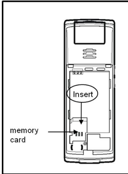
**Figure 19: Installing the MEM card**
