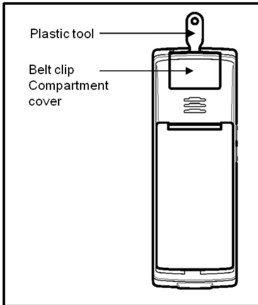
**Figure 14: Using plastic tool**
