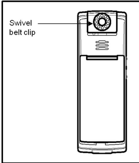
**Figure 15: Installed swivel belt clip**
