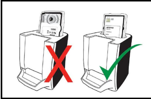
**Figure 4: Placement of I755 spare battery pack**
