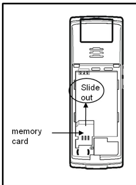
Figure 20: Removing the MEM card
