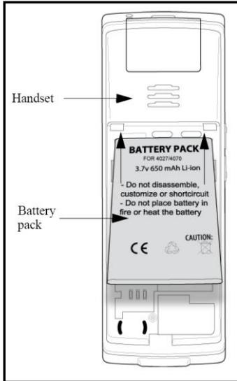
**Figure 1: Installing the G355/G955 battery pack**
