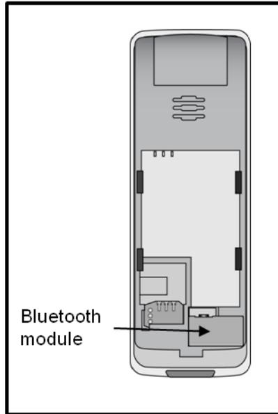
**Figure 21: Bluetooth module installed**
