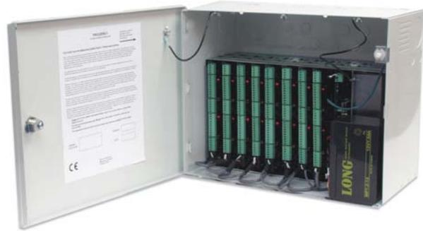
The PRO2200 professional series family of access control modules is connected to the intelligent control module through a supervised RS485 bus at 38,400 bps. Hardware interface configuration options are stored in the intelligent control module and may be directly controlled via operator intervention, time schedules or event-based procedures. The access modules have been designed to allow for a modular customizable solution.
