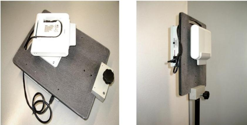
Figure 10. Mounting the Cable between the Battery Cabinet and the Base Station.
