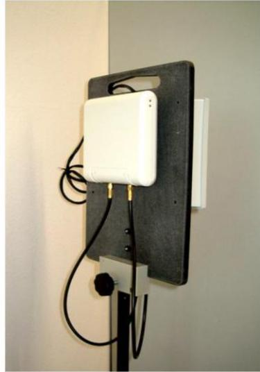
Figure 12. Directional Antenna mounted.
