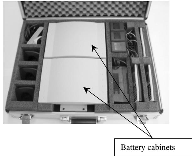
Figure 4. Battery Cabinets in the Site Survey Kit.
