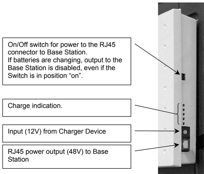
Figure 5. Controls on the Battery Cabinet
