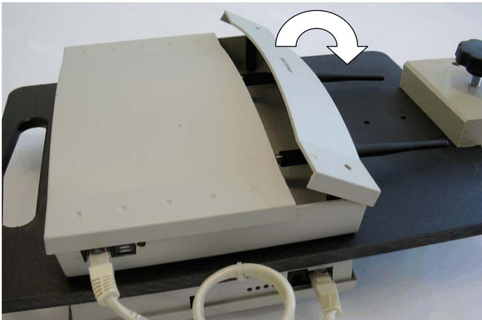
Figure 9. Removing the cover from the Base Station.
