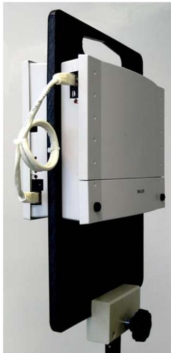
Figure 8. Mounting the Cable between the Battery Cabinet and the Base Station..
