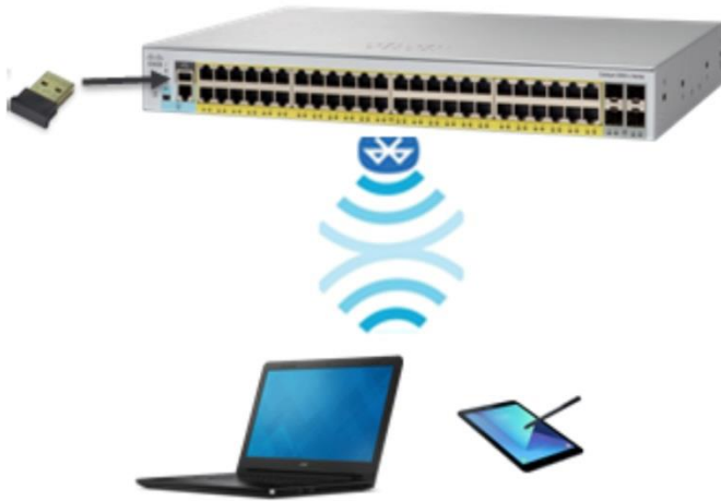
Figure 4. Over-the-air switch access using Bluetooth
