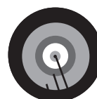
tight-buffered fiber (900 μm buffer) inner tube aramid yarn outer jacket
