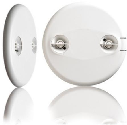
Wattstopper's UT-300 Ultrasonic Ceiling Sensors automatically turn lighting on and off based on occupancy. The sensors mount on the ceiling with a flat, unobtrusive appearance and provides 360° coverage.
