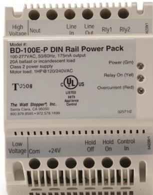
The BD-100 is a versatile, DIN rail mounted power pack supplying 24 VDC operating voltage to low voltage occupancy sensors and other lighting controls. The BD-100 is available in two models, the BD-100E-P with hold-ON and hold-OFF functions, and the BD-100M for manual-ON applications.
