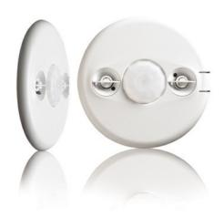
Wattstopper's low profile DT-355 dual technology occupancy sensor combines the benefits of passive infrared (PIR) and ultrasonic technologies. The sensor mounts on the ceiling with a flat, unobtrusive appearance and provides 360 degrees of coverage.
