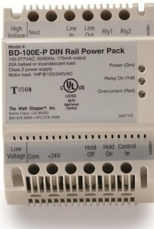
The BD-100 is a versatile, DIN rail mounted power pack supplying 24 VDC operating voltage to low voltage occupancy sensors and other lighting controls. The BD-100 is available in two models, the BD-100E-P with hold-ON and hold-OFF functions, and the BD-100M for manual-ON applications.
