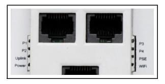
The status lights provide the following information while the MSM317 attempts to discover and establish a management tunnel with an MSM7xx Controller. See *Working with Controlled APs* in the *MSM7xx Controllers Management and Configuration Guide* for more information about the discovery process.
